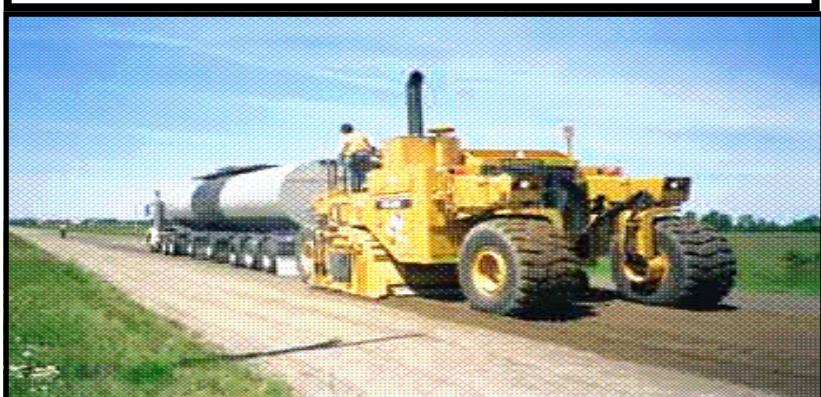
**PZ-22X** can be applied with conventional excavation, graders, water trucks and rollers. However, both deteriorated asphalt and dirt roads can be efficiently recycled/rebuilt using existing material and combining PZ-22X in one process using the tandem recycling unit shown above. **Approved by Alabama DOT.**
